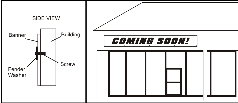
Wall Installation ("Screw & Washer" Method)
